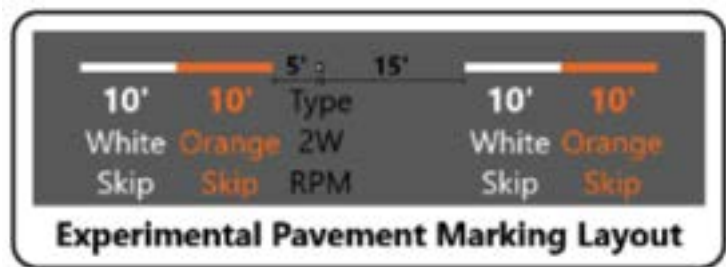
Figure 1. WSDOT Orange Marking Configuration
